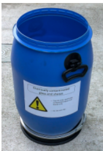
Chemically contaminated glass and sharps bin
