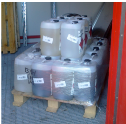
Containers stacked on pallet in fire rated container
